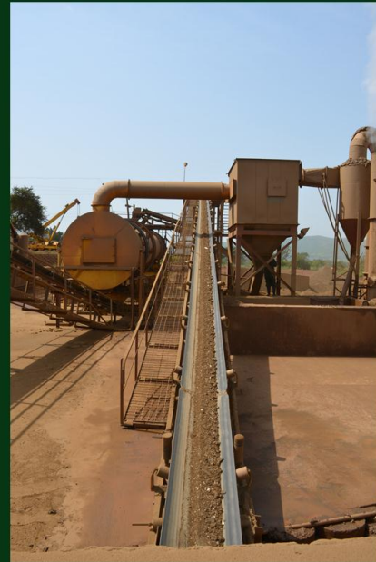
Figure 5. The Namakera Processing Plant – rotary dryer and dryer feed and discharge (Source Namakera Mining Company)
