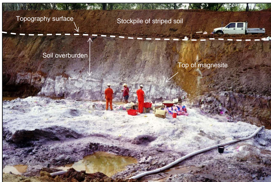
Figure 7 Drill-blasting of exposed magnesite rock in the test pit during the wet season – notice very thin soil overburden
