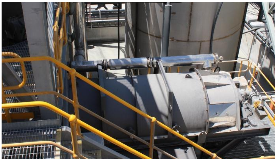
Carbon Regeneration Kiln in operation
