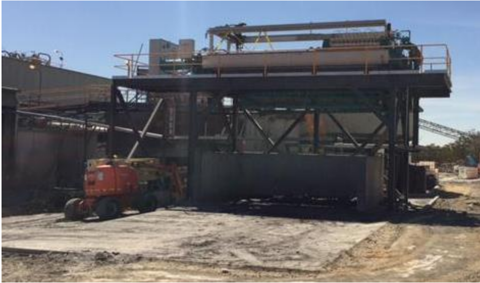
Second Concentrate Filter in operation
