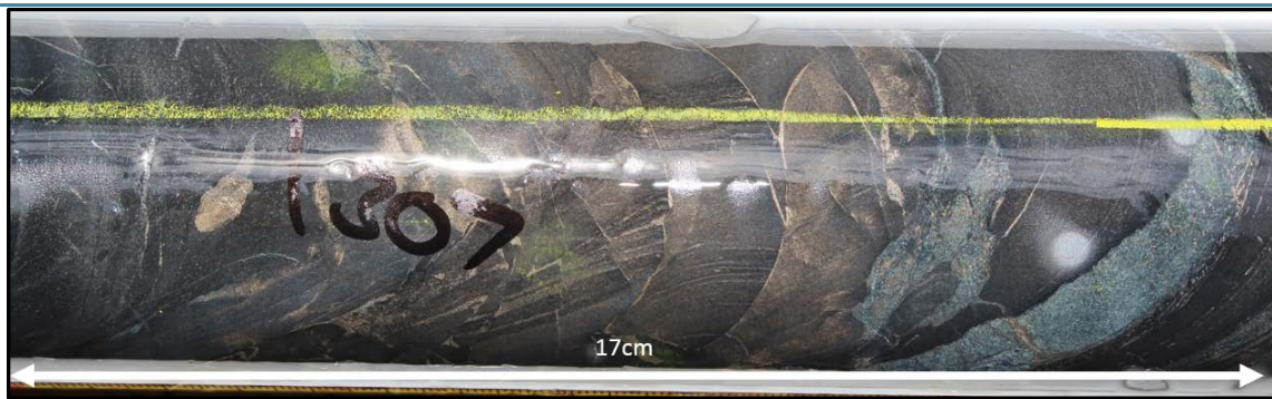
Figure 2 – core from hole MCPDH0002 – 307.00m – semi massive pyrrhotite and minor sphalerite within shale and interpreted volcanoclastic sediments.
