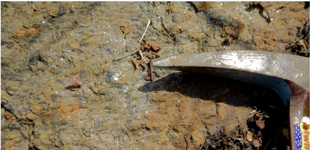
Photo 2, above. Cm-scale aggregate of graphite flakes in hand specimen. Photo 3, below showing finer flake graphite.
