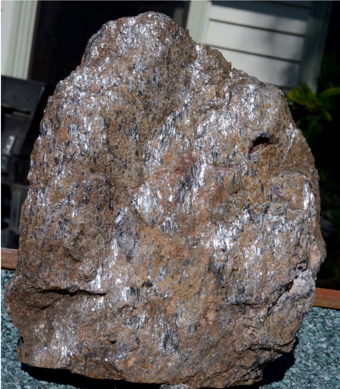
Photo 2, above. Cm-scale aggregate of graphite flakes in hand specimen. Photo 3, below showing finer flake graphite.
