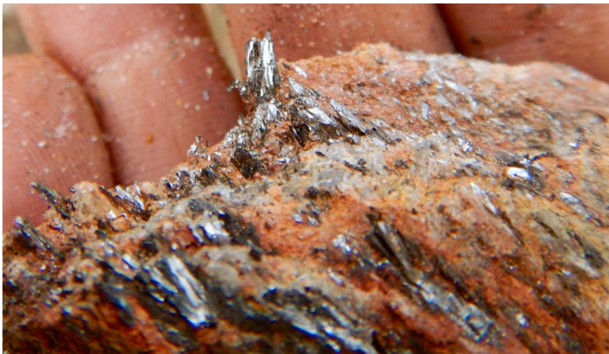
Photo 1. Close-up photo of coarse graphite crystals within surface outcrop at Central lode
