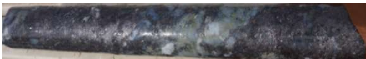
High grade zinc sulphide (sphalerite – bronze metallic coloured mineral)
