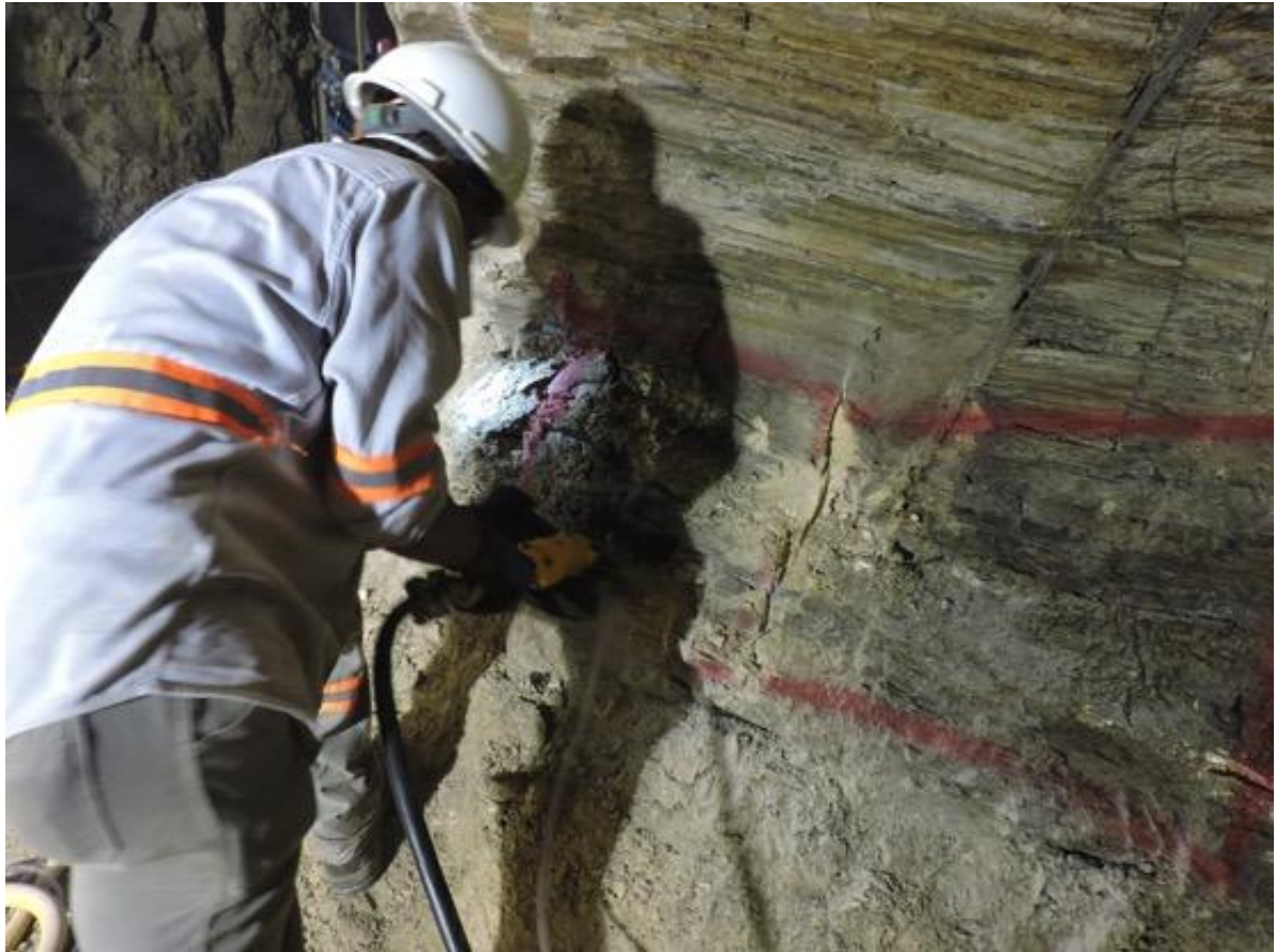
Figure 5. Collecting panel samples from a marked-up wall of a level drive.
