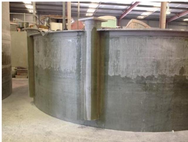
FRP leach tank top section during manufacture
