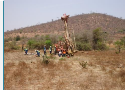
RC drilling – Jubilee Reef Project
