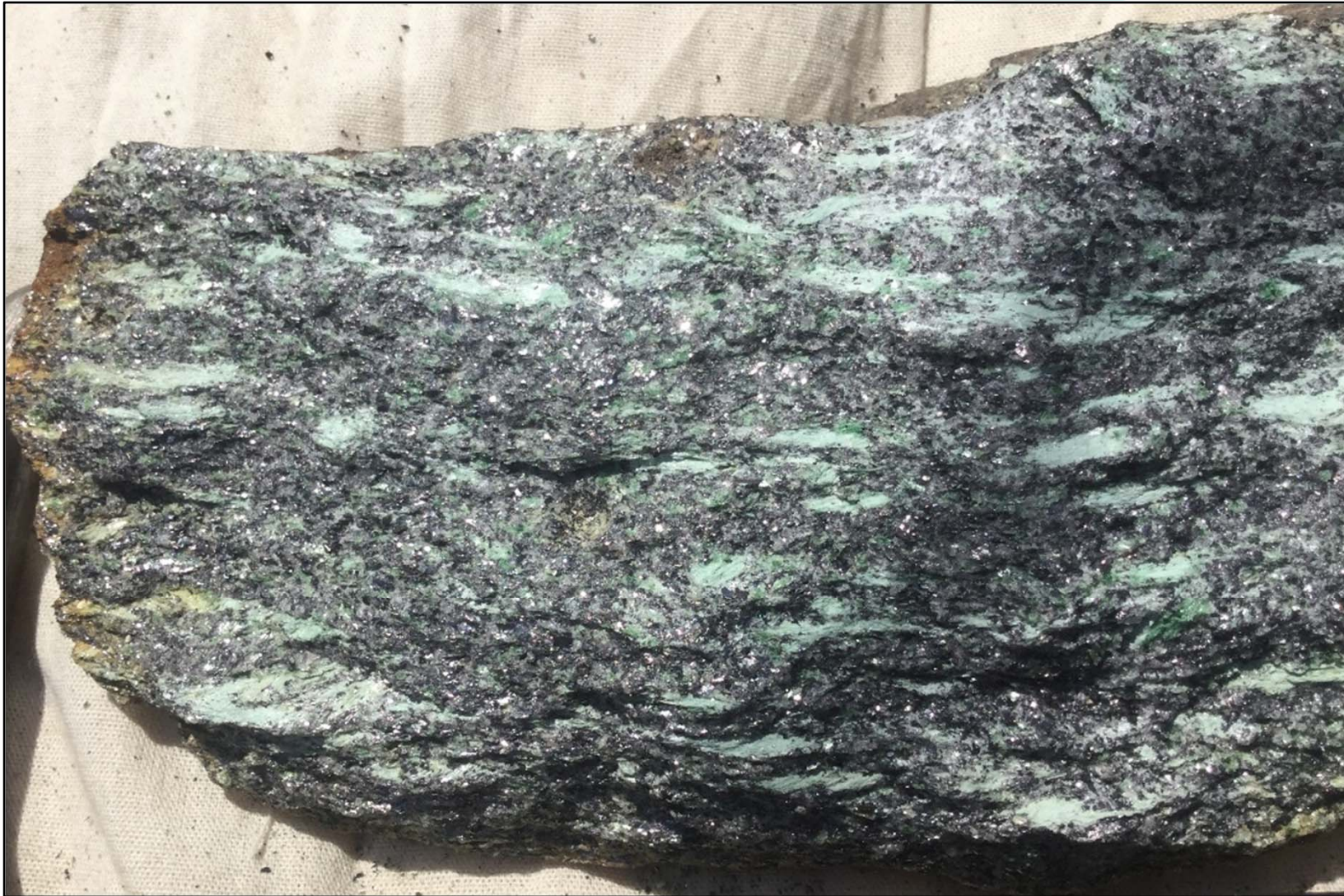
Graphite-Sericite-Quartz Schist 15 – 20% VGE with coarse flake material up to 3mm observed in hand-sample
