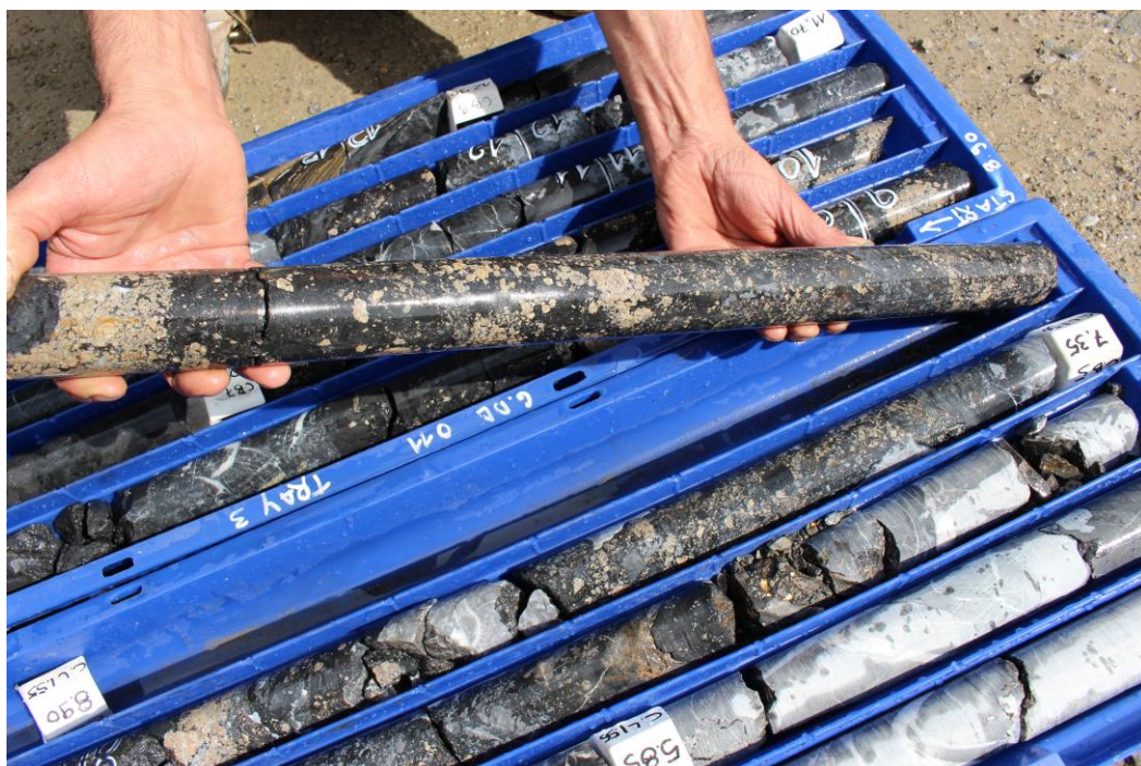
Figure 1: High-grade stratabound zinc sulphides in GDD011 – assays awaited
