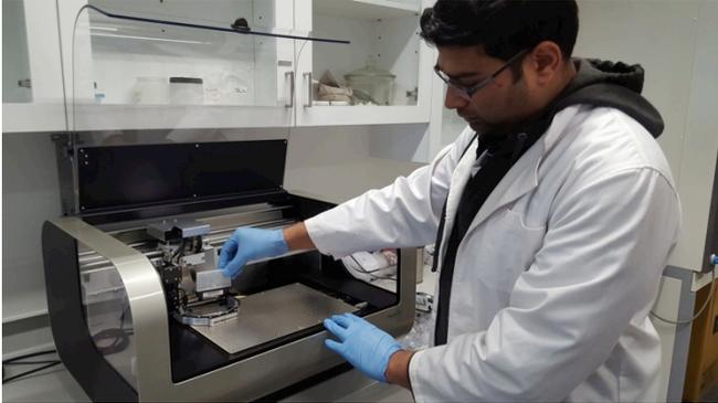
Nanocube ink cartridge being inserted into a Fujifilm Printer
