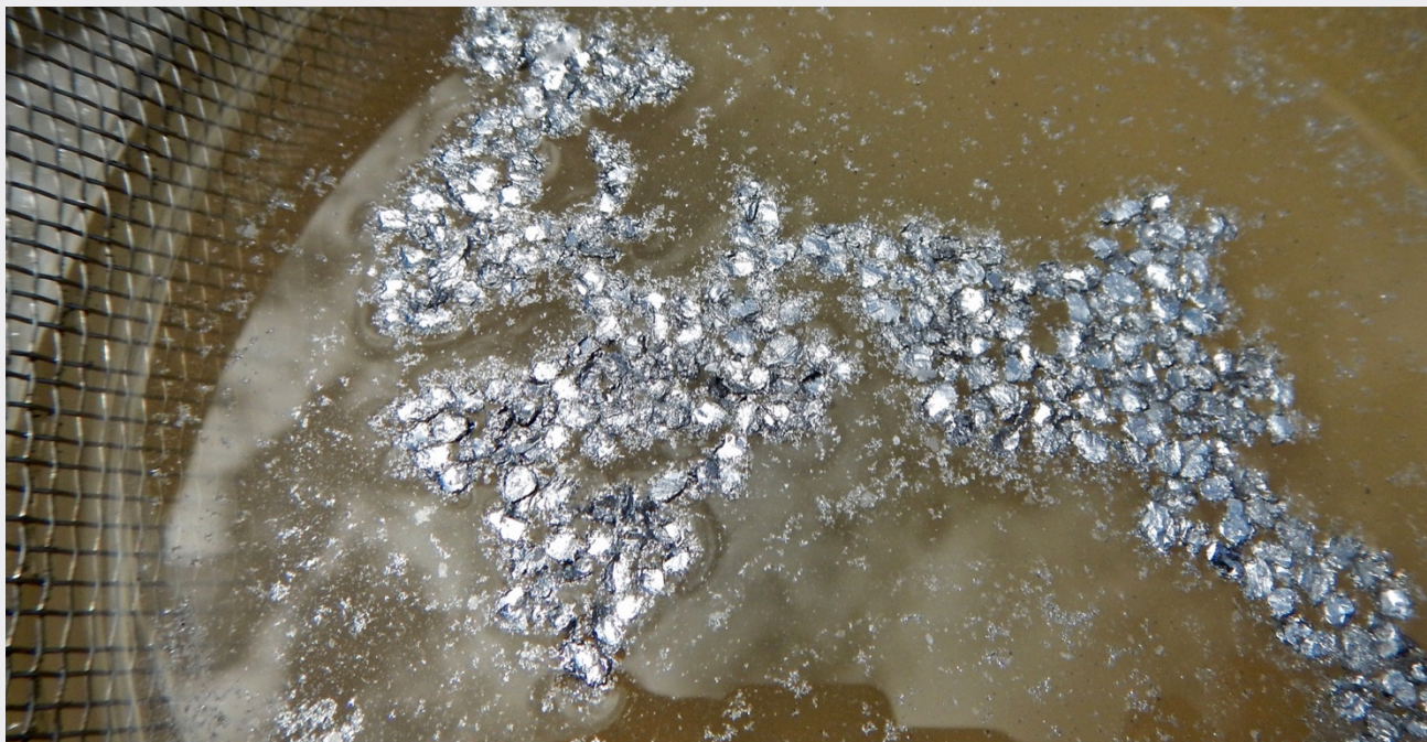
Coarse graphite flakes floating on water at Epanko northeast.
