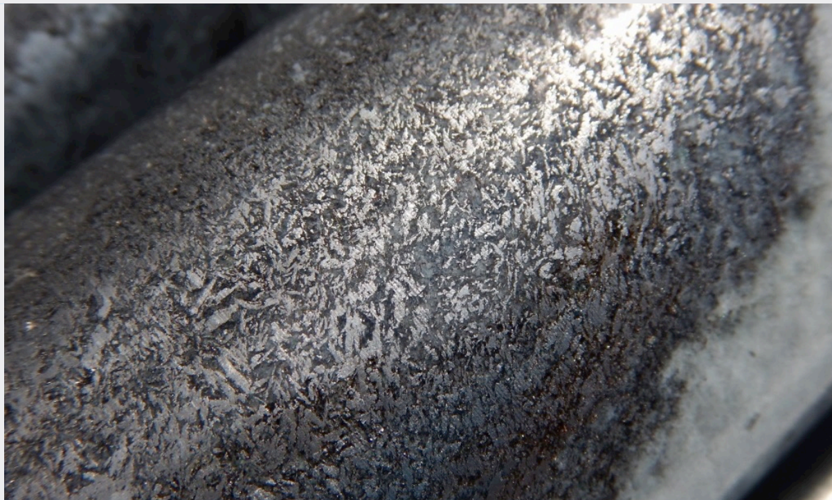
Core from DD14, the first diamond hole drilled at Ulanzi, showing spectacular intergrowths of coarse flake graphite in core.
