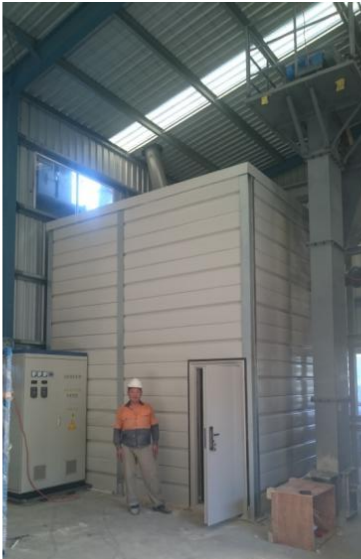
Image 3: Fine Grinding Mill Sound Proof Room.
