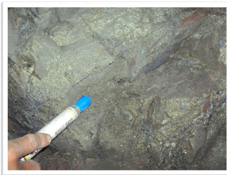
Photo 3: Brasil vein I Sublevel 0, SE. Massive chalcopryite with bornite and pyrite
