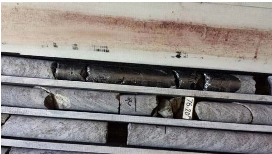
Figure 4: 50 cm graphite vein intersected by AK 04
