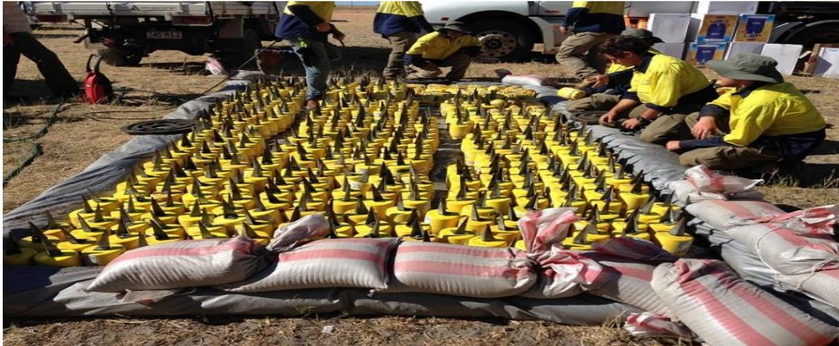
*Figure 4. Terrex cable free nodes being prepared to be placed in the field, EP413 3D Seismic Survey April 2015*
