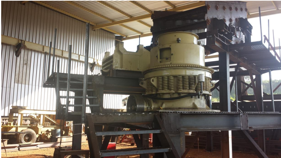
100tph cone crusher in workshop – nearing completion
