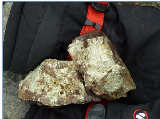
**Figure 2:** Examples of massive chalcopyrite copper ore from Pahtohavare. Samples, likely from the Southern Deposit, were located on the mines' waste dump during a recent field trip.
