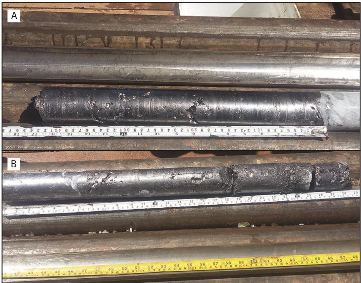
**Figure 9: Graphite core recovery from PLB004. A) Multiple graphite zones up to 6 cm thickness. B) Example of single graphite vein**
