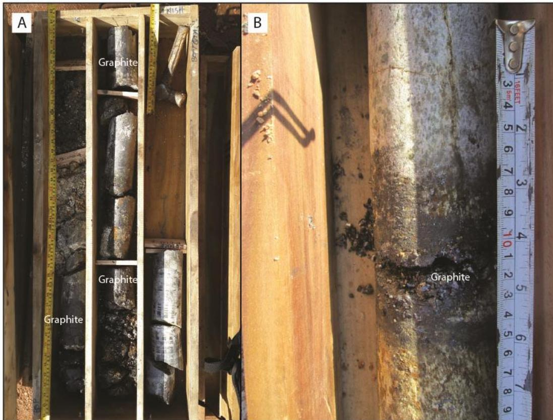
**Figure 8: Graphite core recovery from PLB004 at 52 to 56 m downhole. A) Multiple graphite zones up to 6 cm thickness. B) Example of single graphite vein**
