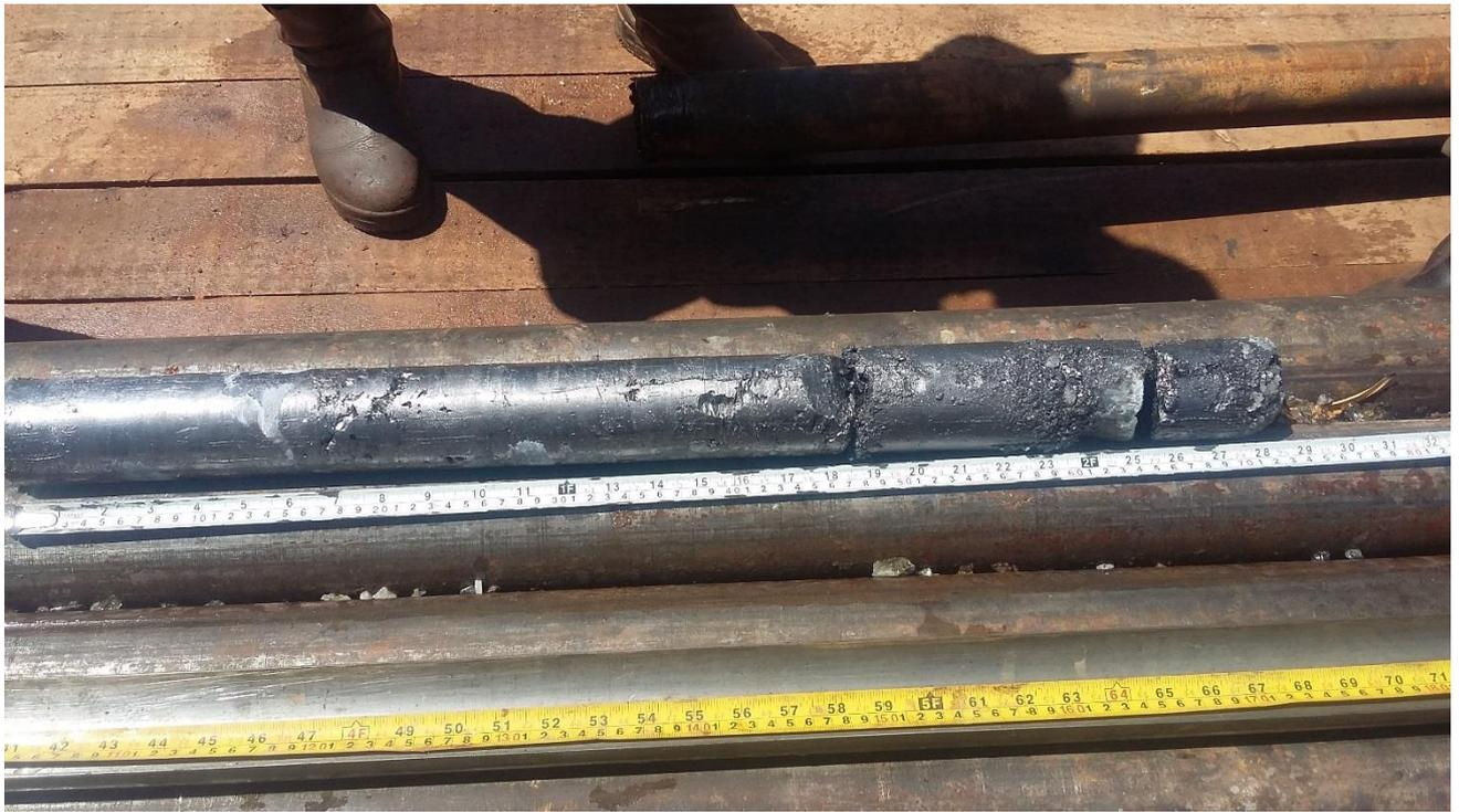
**Figure 1- Graphite core recovery from PLB004 at 89 to 102 m downhole. A thick and continuous graphite intersection.**
