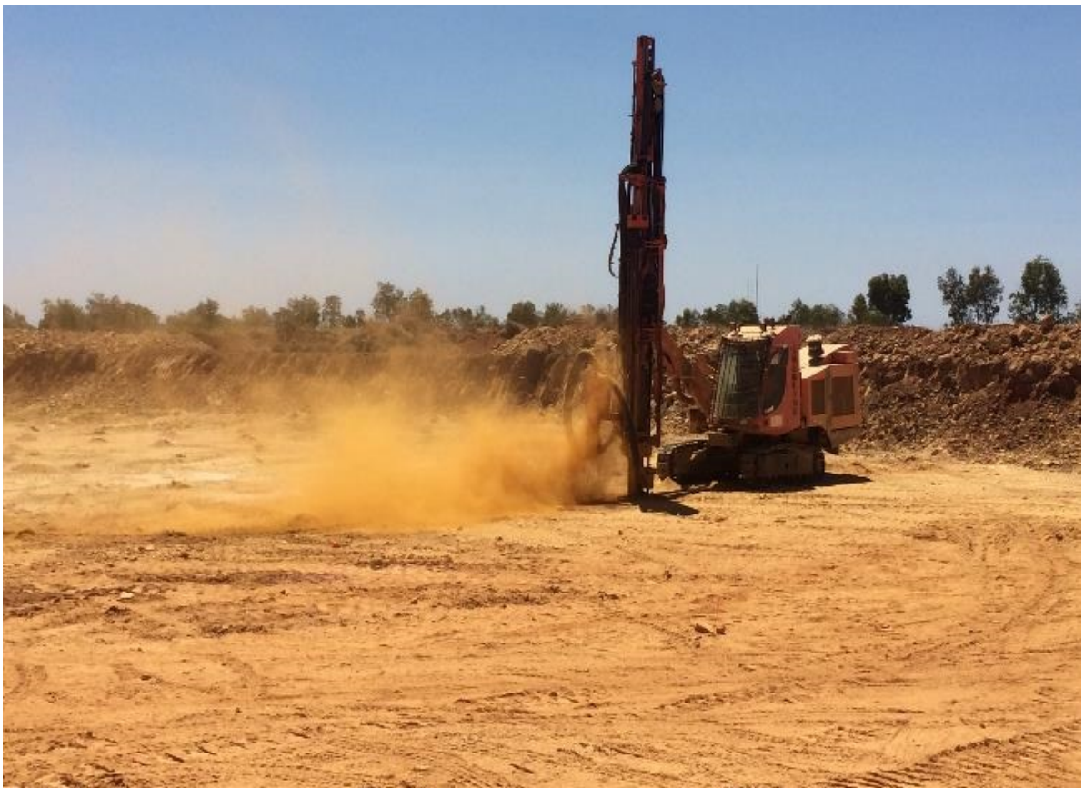
Figure 4. Blast-hole drilling at Golden Hind
