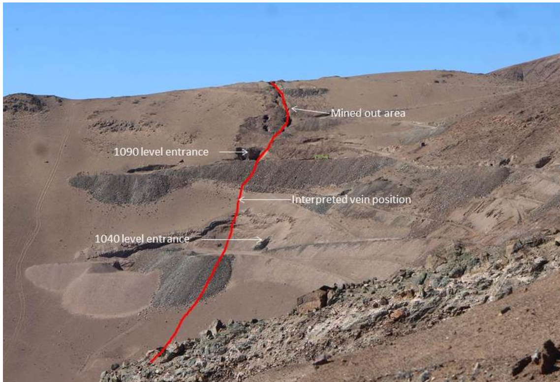
Figure 2 – San Sebastian mine and vein looking north. Note favorable topography for access, vertical distance between the 1040 level and 1090 level entrances is approximately 50m. Work is planned to establish additional mining access tunnels into the vein below the 1040 level.
