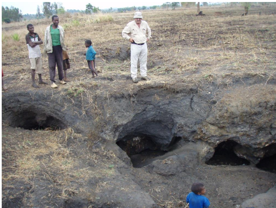
Figure 9. Photograph of high grade graphitic saprolite “chiziro” pit mined by local villagers to produce a graphite concentrate to make paint for their mud brick huts. Rock chip results from these workings assayed 22.4%, 17.1% and 7.7% TGC.
