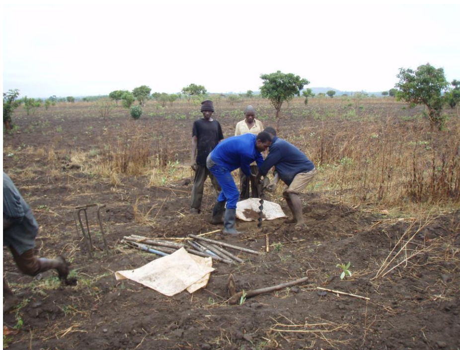
Figure 5. Hand augering in progress at Lifidzi.
