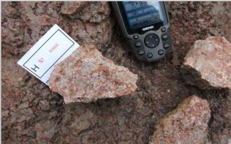
Bauxite sample 63.79% \text{Al}_2\text{O}_3
