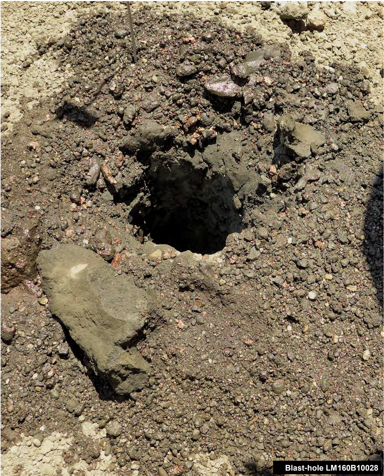
Figure 8: Drill-chip samples from blast-hole drilling are collected through a cyclone splitter on the RAB rig, however not all of the sample makes it to the cyclone, as can be seen in the above image. The Company views this scenario as a hidden bonus to the upside.
