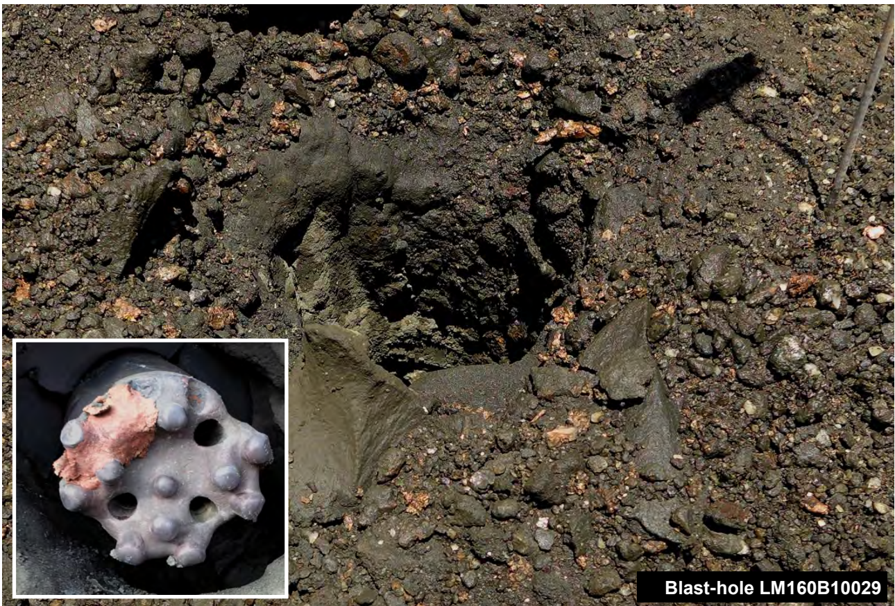
Figure 1: Drill collar of a completed blast-hole, drilled by a Rotary Air Blast (RAB) rig (main image) and native copper stuck on the end of the RAB drill bit (inset). Drill-chip samples from blast-hole drilling are collected through a cyclone splitter on the RAB rig, however not all of the sample makes it to the cyclone, as can be seen in the above image. Comparative analysis of the drill "spoils" versus collected sample indicates a possible underestimation of copper content in samples collected from open-hole RAB drilling in coarse native copper zones. Similar issues were identified at Rocklands during resource drilling in coarse native copper zones using Reverse Circulation (RC) rigs. The Company views this scenario as a hidden bonus to the upside.
