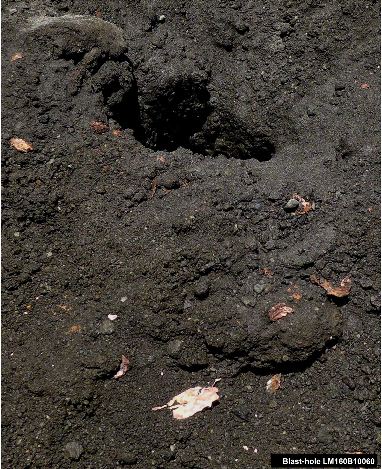
Figure 10: Drill-chip samples from blast-hole drilling are collected through a cyclone splitter on the RAB rig, however not all of the sample makes it to the cyclone, as can be seen in the above image. The Company views this scenario as a hidden bonus to the upside.
