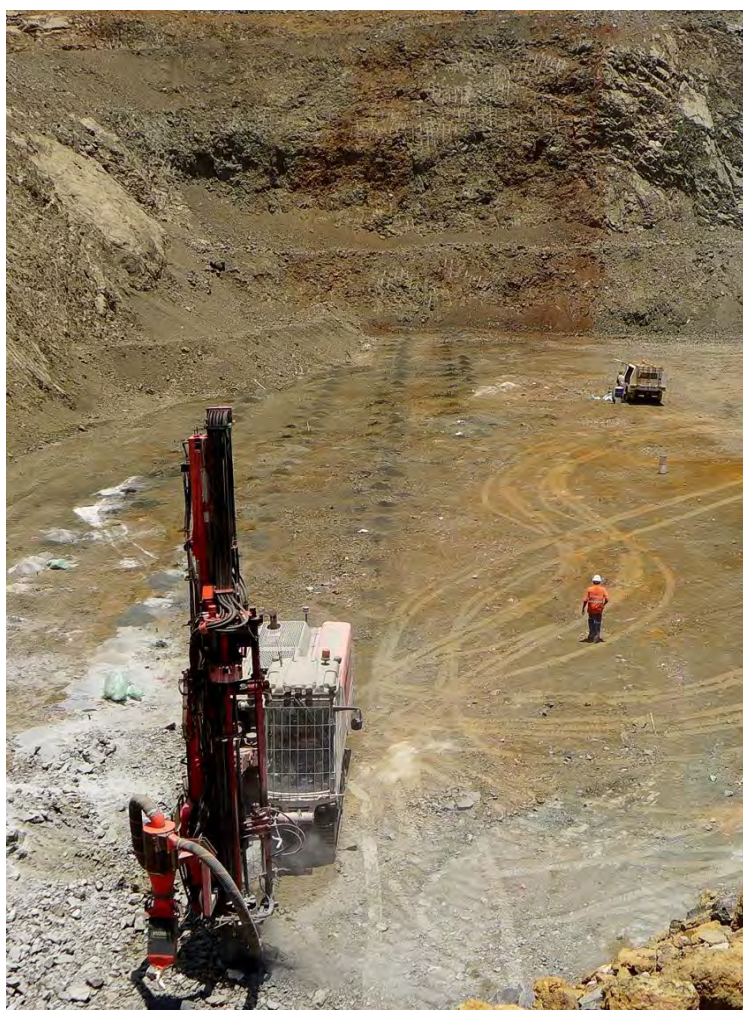
Figure 4: Blast-hole drilling in LM1 Pit. The high-grade native copper ore zone can be easily seen in the pit wall (background).
