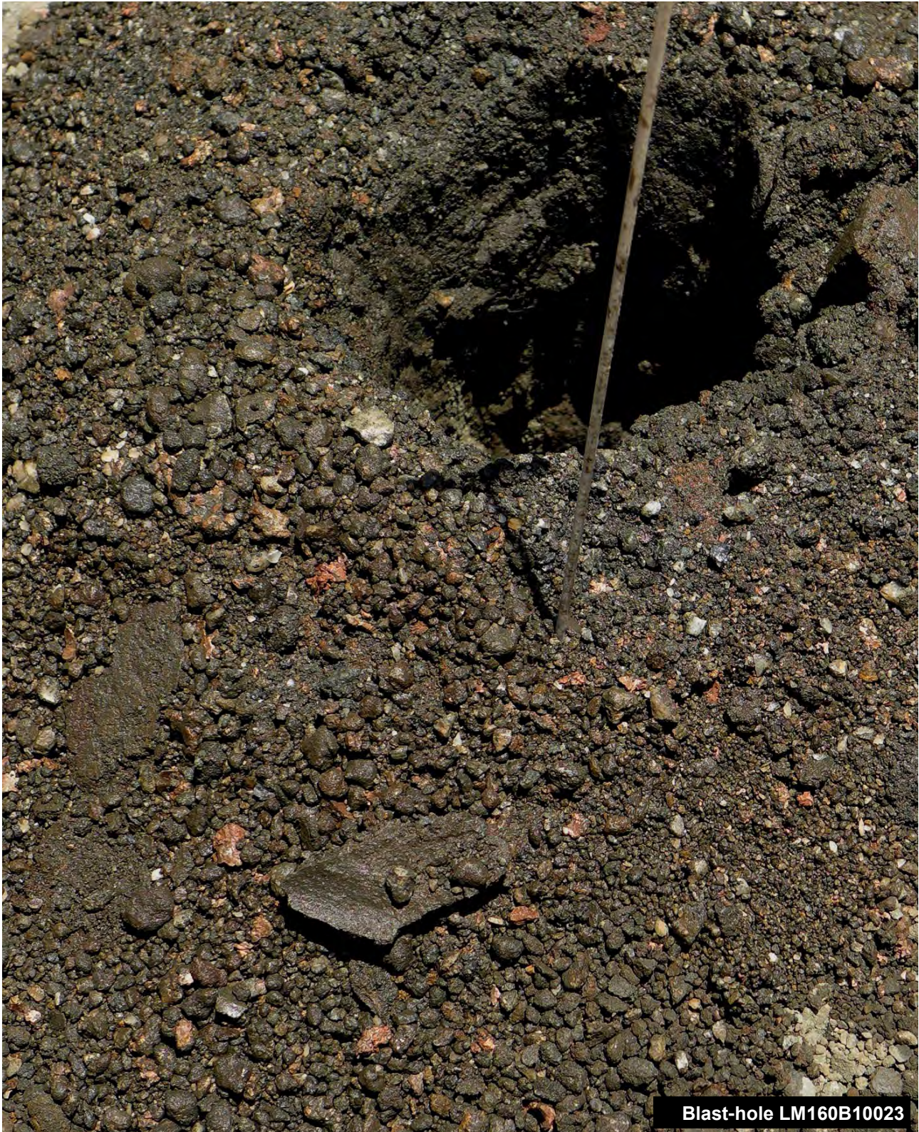
Figure 9: Drill-chip samples from blast-hole drilling are collected through a cyclone splitter on the RAB rig, however not all of the sample makes it to the cyclone, as can be seen in the above image. The Company views this scenario as a hidden bonus to the upside.
