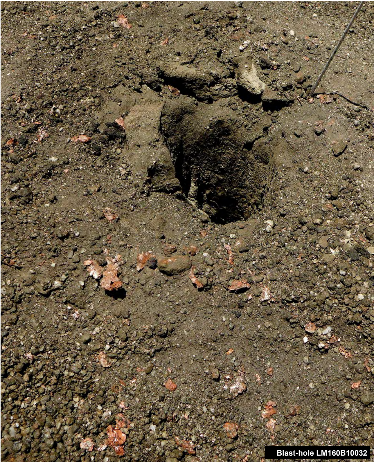
Figure 7: Drill-chip samples from blast-hole drilling are collected through a cyclone splitter on the RAB rig, however not all of the sample makes it to the cyclone, as can be seen in the above image. The Company views this scenario as a hidden bonus to the upside.
