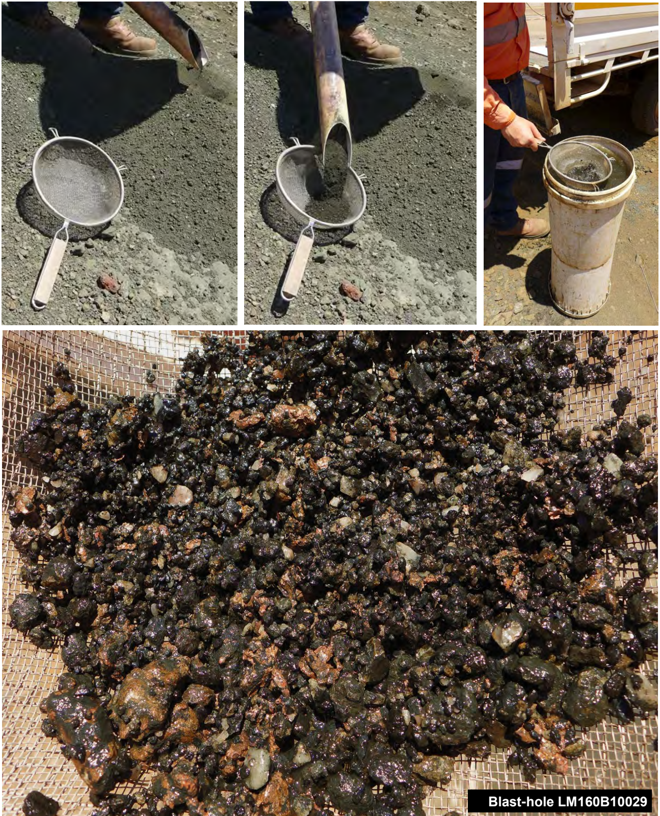
Figure 2: Samples are speared from the blast-hole samples ejected from the cyclone splitter, and used for geological logging. This sample is visually estimated at over 50% copper by weight.
