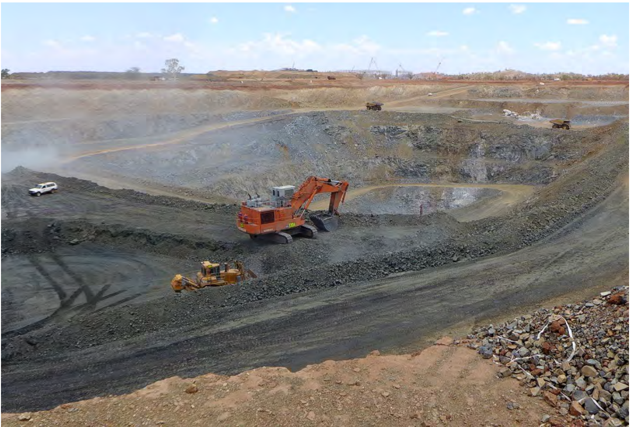
Figure 3: Top image shows the various pit stages at Rocklands that resulted from optimisation with a focus on maximising project Net Present Value (NPV). The below image shows the LM1 Pit recommencing in the middle of the larger LM2 pit that has been the focus of recent mining.
