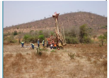
RC drilling – Jubilee Reef Project
