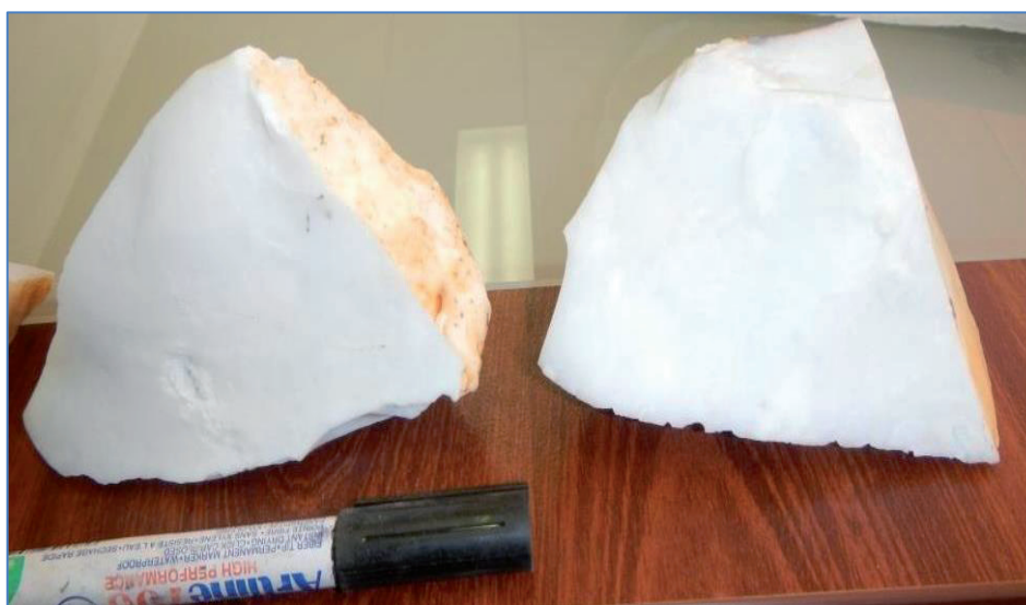
Figure 17. Visually-selected Dingo Hole Silica from outcrop.
