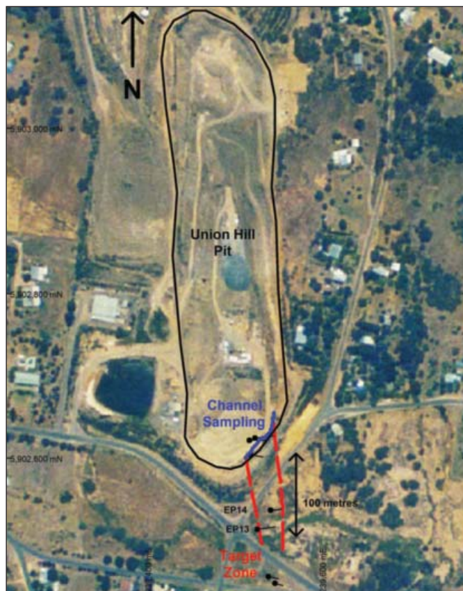
Figure 4 Union Hill open pit with location of pit wall sampling, historic drilling, and exploration target zone
