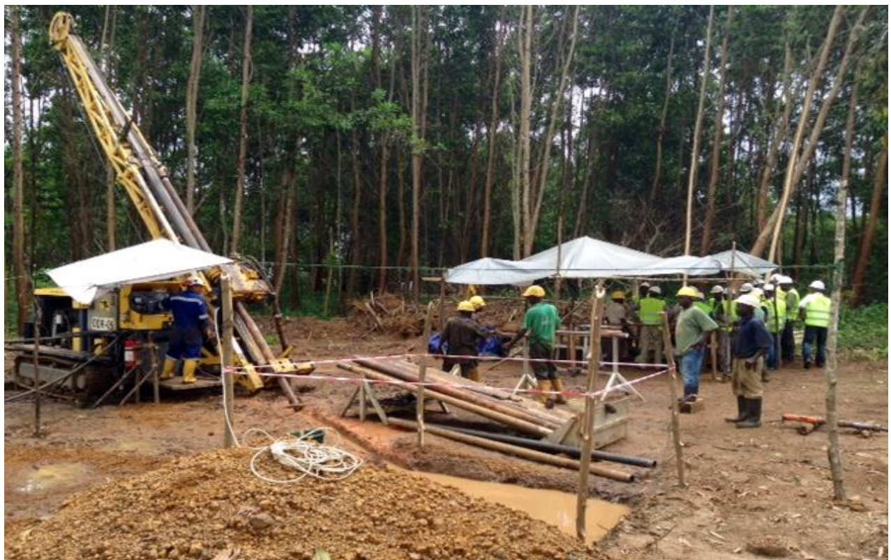
Figure 2 - Diamond drill rig at the Zaway Main deposit.
