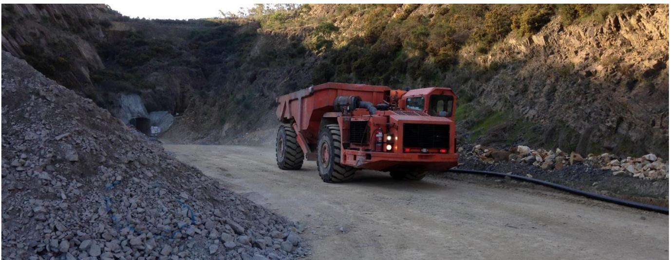
*Recently acquired Toro 45D underground truck carting waste rock from the decline. Scalped pile of low grade ore in left of image.*
