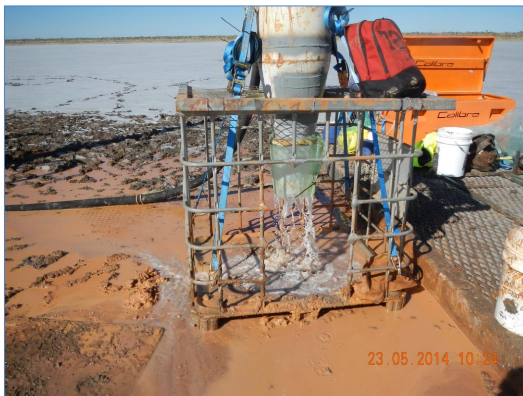
Figure 6. Water flowing through cyclone on LMAC001.
