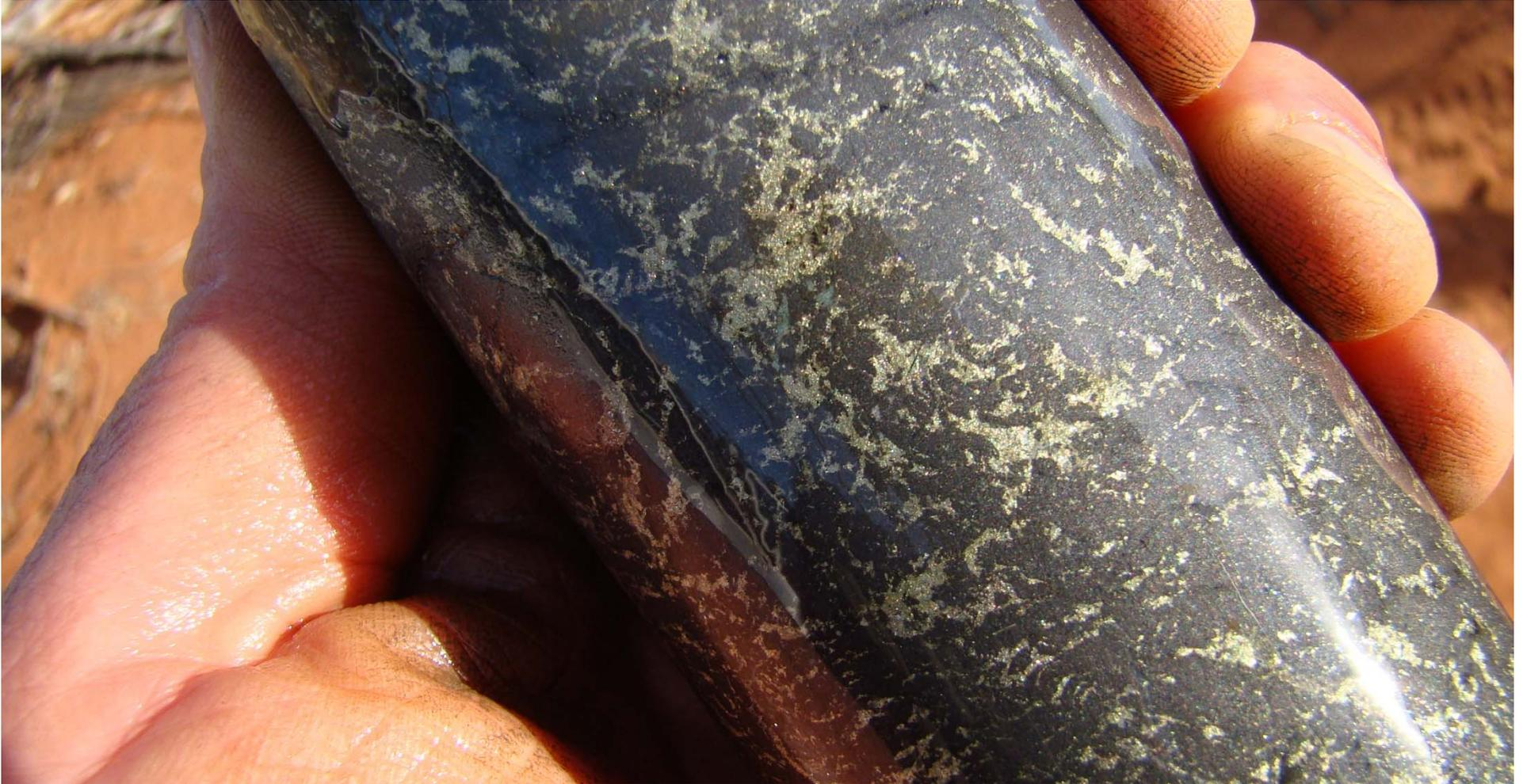
**massive magnetite-copper-gold in brecciated “feeder” structure
