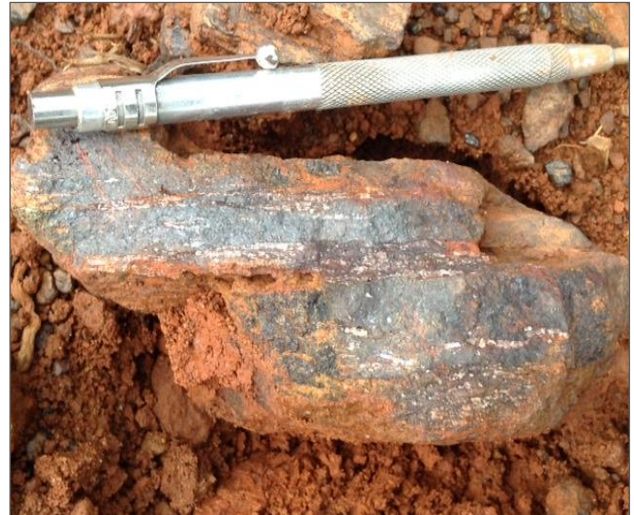
Figures 4 & 5 | Mineralisation in road cutting at Zaway North-West (left), showing shallow dip sub-parallel to surface and (right) high-grade iron mineralisation from cuttings.
