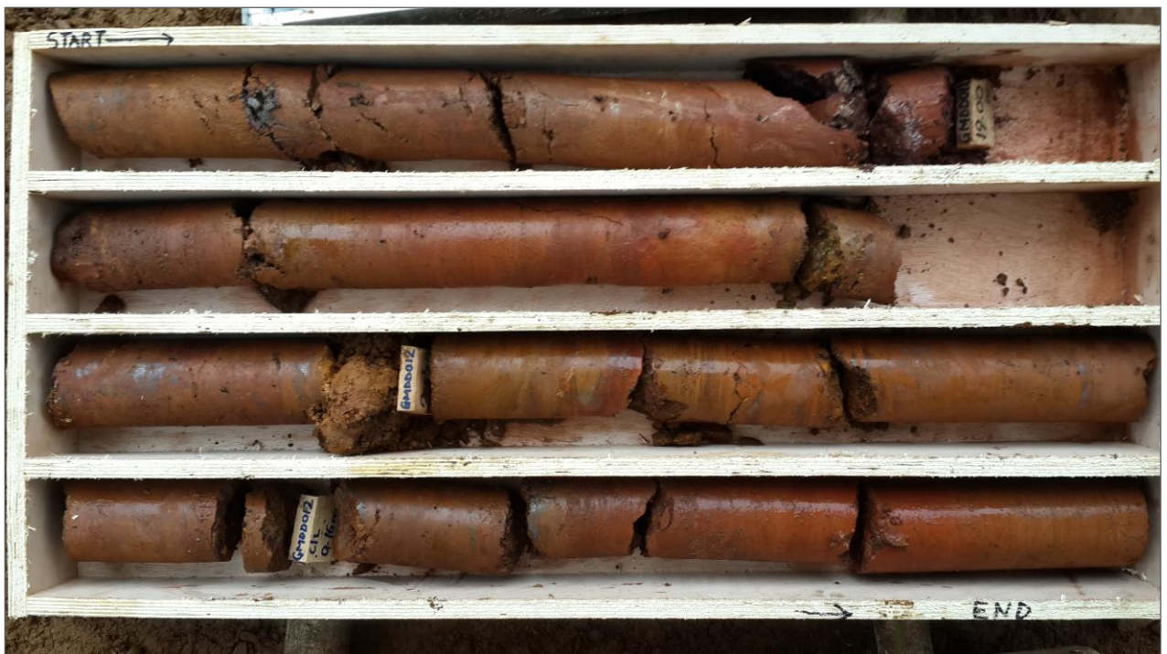
Figure 7 | Diamond drill core recovered from the first drill hole of the PFS programme at the Gofolo Main deposit; high-grade hematite -goethite mineralisation, depth approximately 18-22m down hole.
