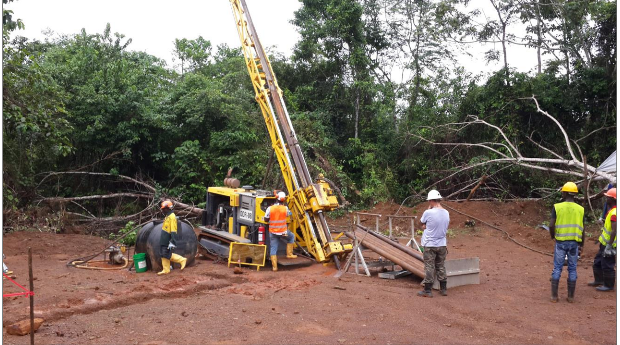
Figure 6 | Diamond drilling currently underway at the Gofolo Main deposit.
